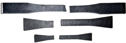
图8 试验件宏观断裂形貌 Fig.8 Macroscopic fracture morphologies of the test specimens
