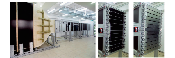
图 8 以色列理工学院的非定常风洞 [7] Fig.8 Unsteady wind tunnel at the Technion-Israel Institute of Technology [7]
