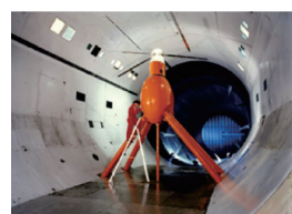
(c) ONERA 7AD model in SMIA wind tunnel [89]
