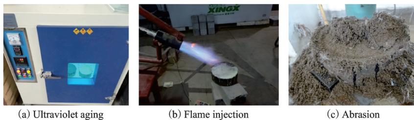
(a) Ultraviolet aging (b) Flame injection (c) Abrasion
