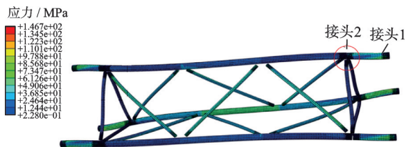
图 17 ZK13-2 梁元等效三角桁架计算结果 Fig.17 Calculation results of ZK13-2 beam element equivalent triangle truss
