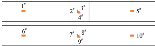
图 4 试件应变具体测量点位示意图 Fig.4 Specific measurement points for strain
