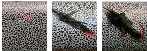
图13 复合材料传动轴弹击损伤情况<sup>[53]</sup>Fig.13 Ballistic damage of composite drive shaft<sup>[53]</sup>
