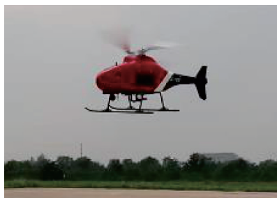
图17 JZ120交叉双旋翼无人直升机 Fig.17 JZ120 intermeshing-rotor unmanned helicopter
