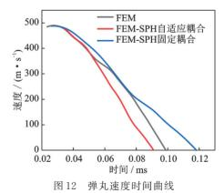
Fig.12 Velocity-time curves of projectile
