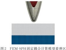
Fig. 2 Impact region of FEM-SPH fixed coupled model
