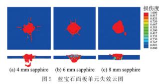
Fig.5 Failure cloud diagram of sapphire panel unit
