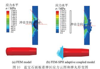
Fig.10 Stress nephogram of the impact zone and the deformation diagram of the projectile on the sapphire panel
