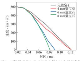
图 6 不同厚度蓝宝石面板弹丸侵彻速度历程曲线 Fig.6 Penetration velocity curves of sapphire panel with different thicknesses
