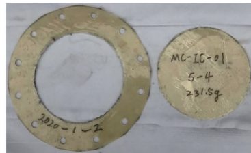
(b) Appearance of frangible cover after breaking
