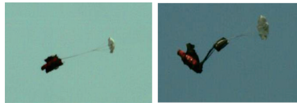
(b1) Departure 0.5 s time (b2) Pilot parachute full time (b) Low speed airdrop dummy picture without control attitude
