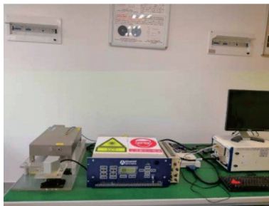
(b) High-rate scanning system
