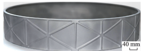
(a) Grid-structure by pass duct casing
