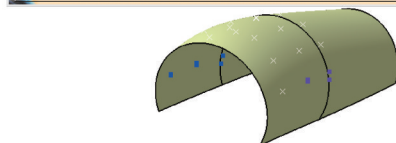
(a) Computation of loading points on fuselage and anomaly detection
