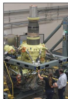
(b) Main gearbox installed on the test bench
