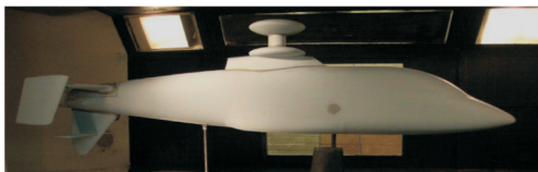
(a) 1/5 scale fuselage model of X2 [43]
