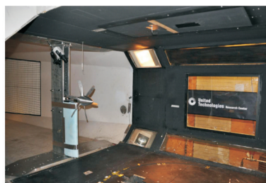
(a) Isolated propeller test [39-40]
