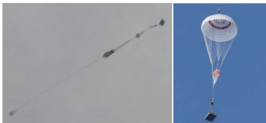
图9 减速伞工作程序 Fig.9 Working procedure of brake parachute
