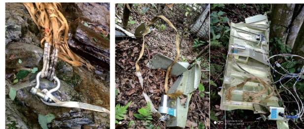
(a) Separation of the lower slings from the brake parachute (b) Lower slings of the brake parachute broken into four and the explosive bolts did not work
