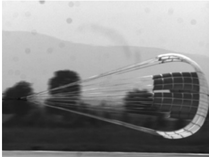
图 4 伞衣完全张满 Fig.4 Inflated canopy
