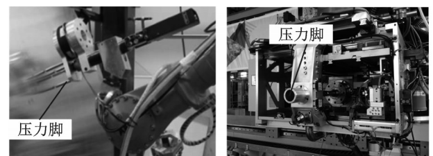
图5 典型刚性压力脚结构 Fig.5 Typical rigid pressure foot
