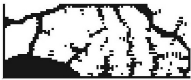
图16 动力学拓扑优化后机翼拓扑结构 Fig.16 Wing topology after dynamic topology optimization
