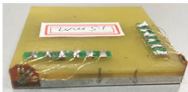
(b) Strain gauges arranged at the corner point
