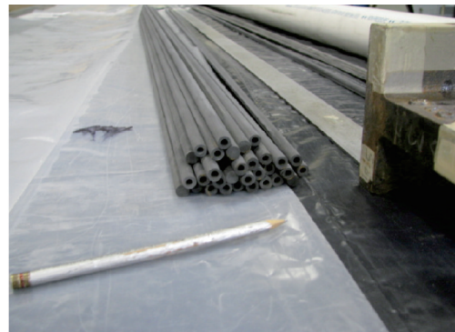
图 17 准备去离子水冲洗的预成型拉挤杆 [57] Fig.17 Preform pultruded rod prepared for deionized water rinse [57]
