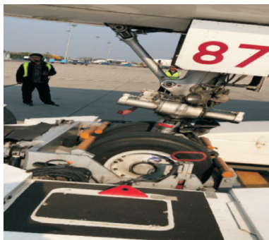
图 10 牵引车顶推飞机工作图 Fig.10 Process of pushing plane
