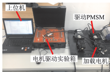
图12 基于ICKF的三相PMSM无传感器控制实验平台 Fig.12 Experiment platform of three-phase PMSM sensorless control based on ICKF
