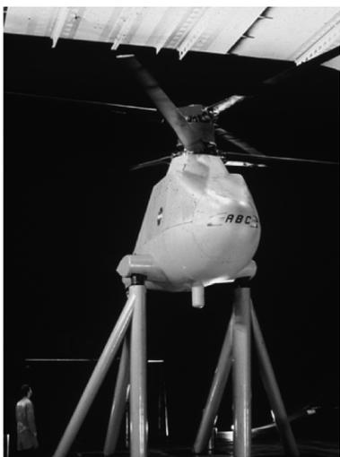
图21 XH-59A全尺寸风洞试验<sup>[28]</sup>
