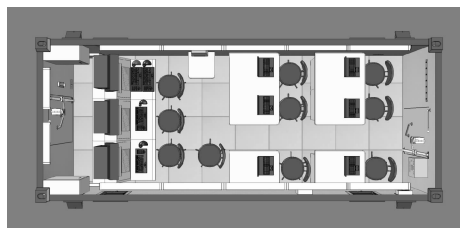
图 4 CZ-6 测发控系统后端电气方舱俯视图 Fig. 4 Top view of CZ-6 rear electrical shelter
