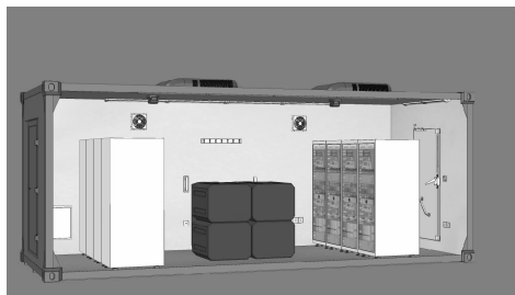
图 3 CZ-6 测发控系统前端电气方舱透视图 Fig. 3 Perspective view of CZ-6 front electrical shelter
