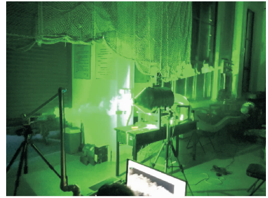
(b) PIV test process
