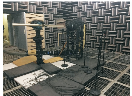
(a) Equipment installation of noise test
