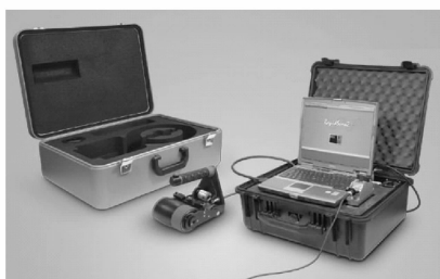
(a) System of Rapid Scan 2 ultrasonic C-scan equipment
