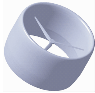
图2 涵道螺旋桨外形 Fig. 2 Ducted propeller shape
