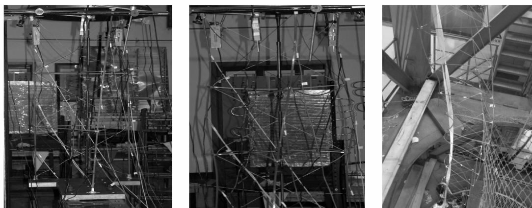
(a) 钢丝绳松弛(3节) (b) 钢丝绳张紧(3节) (c) 钢丝绳张紧(37节)
