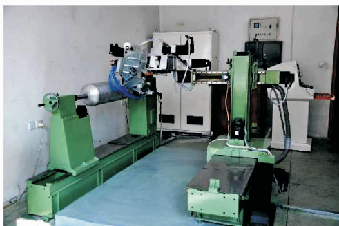
图 13 哈尔滨工业大学 4 丝束自动铺丝原理样机 Fig. 13 Prototype of fiber placement machine with four tows designed of Harbin Institute of Technology
