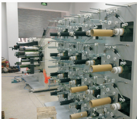
图 16 预浸纱分切-卷绕机 Fig. 16 Split prepreg cut-winding machine
