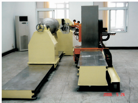
图 12 武汉理工大学 4 丝束自动铺丝原理样机 Fig. 12 Prototype of fiber placement machine with four tows designed by Wuhan University of Technology
