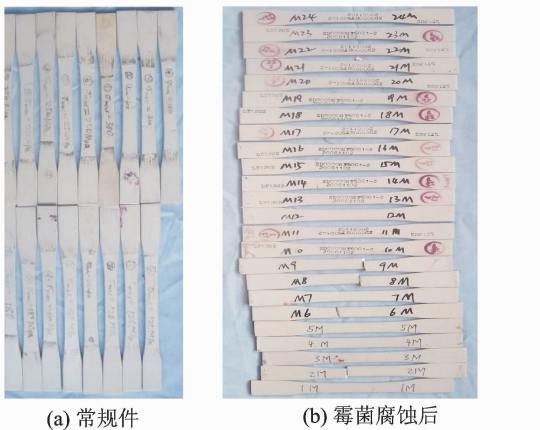
图 3 2A12 试件霉菌腐蚀前后疲劳试验破坏对比照片 Fig. 3 Failure photos of 2A12 specimen before and after fungus corrosion in fatigue test
