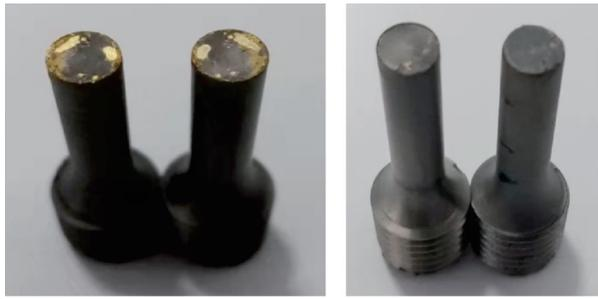
(a) Flame brazing specimen (b) Vacuum brazing specimen
