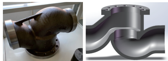
(a) Physical drawing of a three-way valve (b) Modeling profile of a three-way valve
